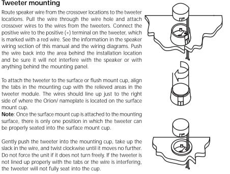
To remove the tweeter, simply turn it counterclockwise, and pull the tweeter away from the cup.
